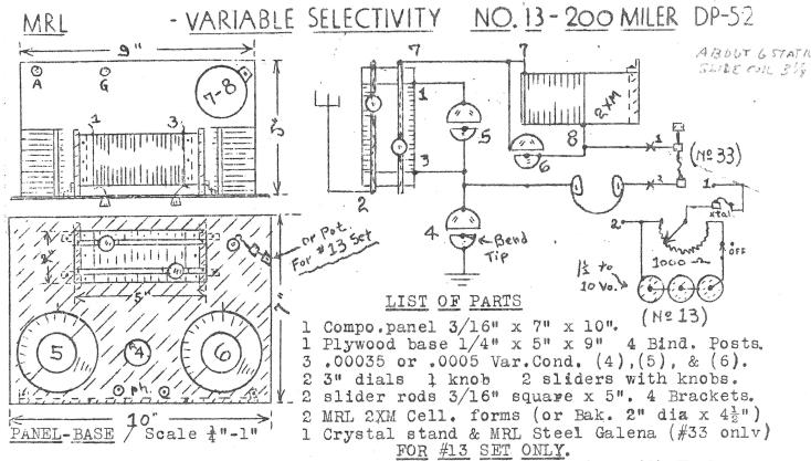
1 MRI Fixed Carborundum Crystal. 1 1000 Ohm Potentiometer with Knob. 1 SPST Panel switch 1 to 4 dry-cells Battery leads, etc.
